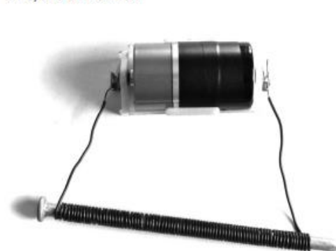
FIGURE L10.3 _____ Electromagnet made from a D-cell battery, a copper wire, and an iron nail
